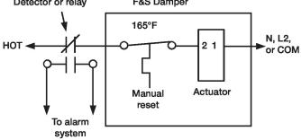
**Parallel Actuator Wiring**
